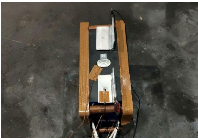
Figure 6. Thermocouple, Film Heater, and Steel Plant Positions
